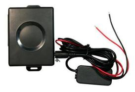
The tracker can also be connected to a car battery using an external power adapter (9-30V input 5V output). Insert the external power adapter output wire to the tracker charging socket and connect the external power adapter input to the car battery (9-30V). Once the battery is fully charged, the tracker will stop charging and use the external power adapter for continued operation, the built-in battery will only be used for backup.
